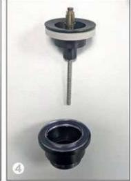
Unscrew the top cover to reveal the brass click-clack bracket. A stainless steel bracket will have also been included within the pack which can be switched with the brass bracket to ensure the waste stays open - usually used for basins without overflows.
