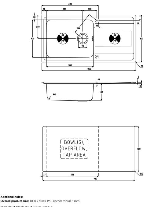
Taphole(s) detail: 2 x Ø 35mm, precut Wastehole(s) detail (mm): 90 / N/A / N/A
