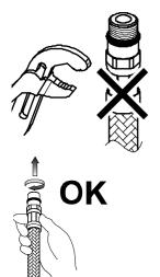
Always screw the flexi hoses into the product only by hand, until feeling mechanical rest, a spanner must not be used on the product end of the connecting hose.
