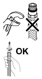
Always screw the flexi hoses into the product only by hand, until feeling mechanical rest, a spanner must not be used on the product end of the connecting hose.
