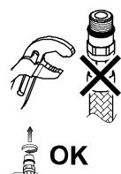
Always screw the flexi hoses into the product only by hand, until feeling mechanical rest, a spanner <u>must not</u> be used on the product end of the connecting hose.
