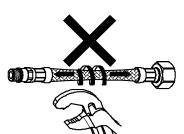
Never twist or stretch the flexible hose during installation.
