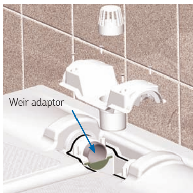
Trap and strainer are removed to give clear access for rodding if required.
