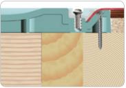
**Clamping strip detail:** Typically floorboards are 18mm thick. It would be necessary to lay plywood on the bathroom floor to bring the floor up to the tray height, for complete level access.
