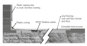
**Step 1.** Position the SureForm over the desired location for the shower. Formers are trimmable and can be cut to down to minimum 150mm to the waste area. Ensure the cut edges are straight and put towards the wall mounted side. If necessary cut to the correct size with a suitable circular saw or a fine toothed blade. Mark around the edge of the shower former.
