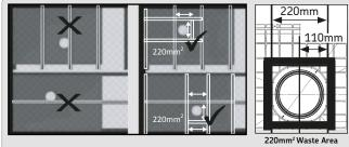
By rotating the rectangular former by 180° the waste position location can be moved to avoid the joists. The waste area must be fully supported with additional joists within 220mm<sup>2</sup> from the centre of the waste outlet area.
