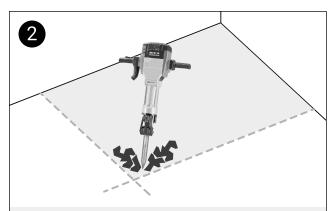
Carefully remove the floor material to a depth of 24 mm. Be aware of any buried cable or pipework.
