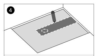
Remove the former. Determine the routing of the waste pipe.
