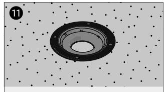
Once the screed base has set, the installation can be continued. Fill the screw holes along the former's edges with a filler.
