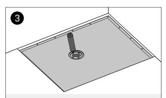
Place the former into the recess, ensuring that it fits neatly. Mark the position of the waste hole.
