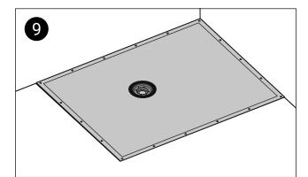
Place the former back into the recess and tamp it down. Ensure that it is level and that the top surface is flush with the floor. Lift the former and add more screed if necessary.
