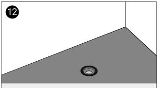
Install the finished floor, e.g. tiles or vinyl flooring. Fit the remainder of the waste.
