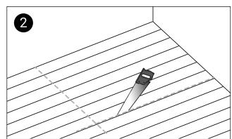
Cut the floor boards, taking care not to cut through the supporting joists or any plumbing or wiring.
