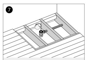
Connect the waste body to the waste pipe. Pack the waste body up to just below its final position.\* Pour some water down it to check for leaks.
