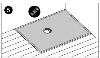
Place the former into recess to determine the waste position and waste pipe routing. Check that the former is level. Remove the former.
