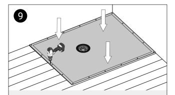
Place the former into the recess and screw it down. Each corner must be screwed down. Screw into joists where possible. Screw down enough to ensure that the former will never move.
