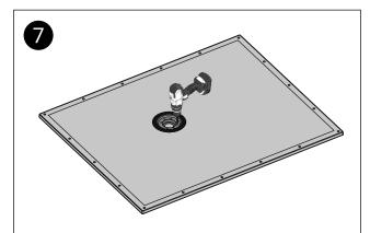
Offer the adapter ring to the former and drill 3.5 mm holes. Attach the adapter ring to the former.
