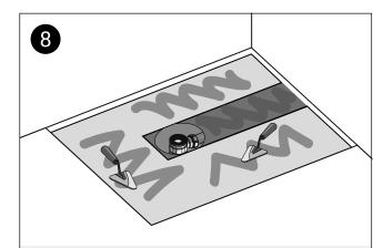
Pour a self levelling screed mix into the recess.
