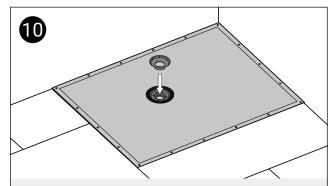
Insert the waste's lock ring into the thread of the waste body. Wind the lock ring into the thread to draw the waste body up. If necessary, use plywood boards to bring the floor up to be flush with the top of the former.
