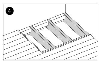
Insert noggins between the joists to support the edges of the former. Perform any necessary packing to ensure that the former is level.
