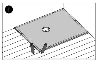
Place the former over the desired location for the shower and mark lines around the edges.
