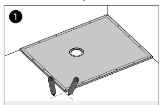
Place the former over the desired location for the shower and mark lines around the edges.
