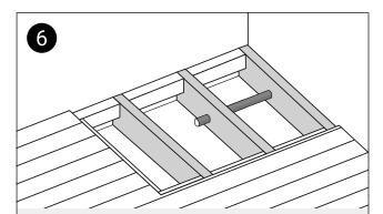
Route the waste pipe. If routing through joists, drill holes. Do not cut notches. The holes in the joists must allow for the upward travel of the waste body (steps 7 and 10).
