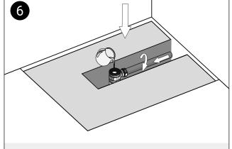
Place the waste body into the recess and connect it to the waste pipe. Pack the waste body up to just below its final position.\* Pour some water down it to check for leaks.
