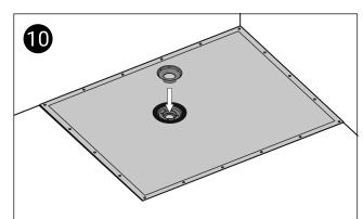
Insert the waste's lock ring into the thread of the waste body. Wind the lock ring into the thread to draw the waste body up.
