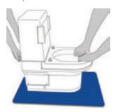
4 Remove self-tapping screw from lower case and face of pan.
