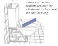
12 To attach Palma Vita to the floor/wall, fix suitable bolts or fixings through the frame and secure the unit in place.
