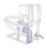
17 Replace cistern cover taking extra care not to prevent the flush function by blocking the flush paddles.
