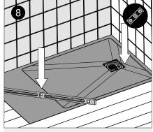
Attach the waste trap to the tray with the waste clamping ring, see separate waste instructions.
