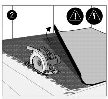
For 'in' floor installation, cut into the flooring, taking care not to cut through any supporting material, plumbing or electrical wiring.
