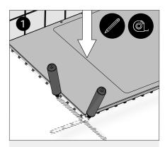
Position the tray over the desired location for the shower and outlet pipe. Mark around the edge of the shower tray and the waste area.
