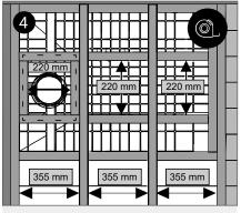
The waste area must be supported with additional noggins, 220 mm around the waste. Additional noggins or joists must be used on all tray edges and between joists centres at a minimum of 355 mm.
