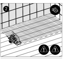
For 'in' floor installation, cut into the flooring, taking care not to cut through supporting joists or any plumbing or electrical wiring.
