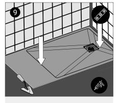
Safety flooring or tiles should finish flush up to the edges of the tray and sealed with sealant. Protect the waste trap from debris during installation.
