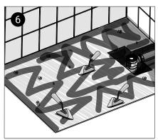
Remove any debris and ensure that there are no sharp edges or raised areas that will affect the tray height. Add 6:1 cement mix to the full tray area and correct height including all supporting edges.
