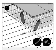
Position the tray over the desired location for the shower and outlet pipe. Mark around the edge of the shower tray.
