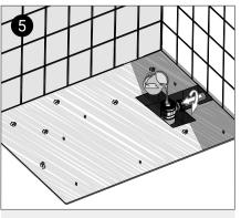
Install the waste drain trap and waste outlet pipe. Water test the waste for flow and for any leaks. Ensure that the rubber seal is in place on top of the trap. Check the waste drain position with the tray.
