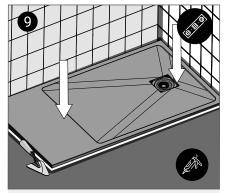
Safety flooring or tiles should finish flush up to the edges of the tray and sealed with sealant. Protect the waste trap and cover from debris during installation.
