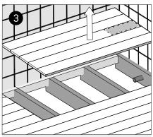
Carefully remove the floor boards and locate the waste outlet pipe. For 'on' floor installation, remove the floor boards around the waste area.
