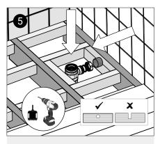
Install the waste drain trap and waste outlet pipe. Do not cut into the joists, always drill through when connecting to the waste outlet pipe.
