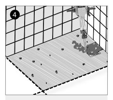
For 'in' floor or 'on' floor installation remove the floor material for the waste area and a channel for the outlet pipe.
