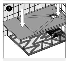
Lower the tray into position and check the height compared to the finished floor height. Firmly secure the tray into position and check all 4 sides are level again.
