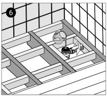
Water test the waste drain trap for flow and any leaks. Ensure that the rubber seal is in place.
