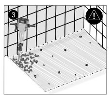
Carefully remove the flooring to suit the finished height of the tray and final floor covering. For 'on' floor installation, remove the material around the waste area.
