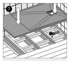
Apply grab adhesive to all the contact points between the tray, joists and noggins. Lower the tray over the waste position and firmly secure the tray into position and check all 4 sides are level again.
