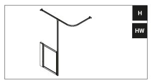
These screens can be fitted to normal trays and trays with integral or optional pipework ducts. The extra wide wall compensators are required for trays with pipework ducts.
