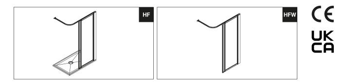
These screens can be fitted to normal trays and trays with integral or optional pipework ducts. The extra wide wall compensators are required for trays with pipework ducts.
