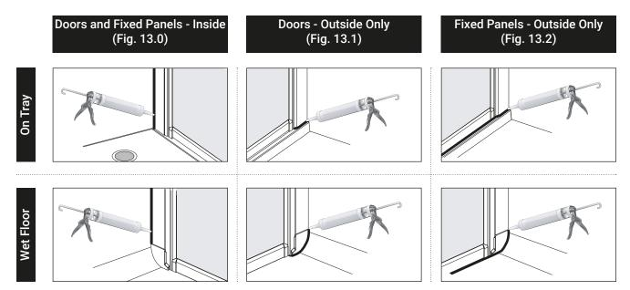
On the outside of the screen, apply silicone sealant along the bottom of the compensator or corner block (for wet floors) and along the bottom of the fixed panel.
