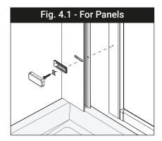
Slide the door or panel into the compensator. Re-attach the adjustment mechanism and loosely tighten the clamping plate using a  $3.5 \times 19$  mm pan head screw (No.6 x 3/4"). Note - Illustrations viewed from inside of tray.
