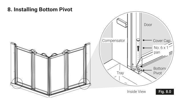
Drill a 3 mm pilot hole for the bottom pivot's screw and fasten using a  $3.5 \times 25$  mm pan head screw (No.6 x 1"). Insert the screw cover cap.
