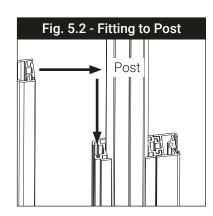
For a panel, overlap the extrusions and slide it down the post (Fig. 5.2). For a door, apply a thin layer of clear silicone to the mating face of the bottom pivot block. Attach it with a  $3.5 \times 25$  mm pan head screw (No.6 x 1") and then slide the door down the post. Fig. 5.2 shows fitting to an inline post. The process is the same for fitting to a corner post.
