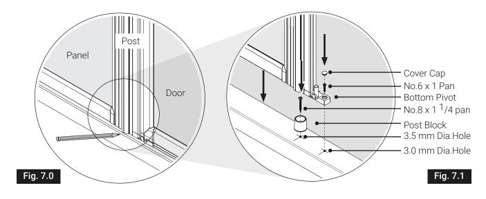
Mark and drill the screw hole positions (Fig. 7.1). NB, the holes are different sizes. Screw the post block down with a  $4.2 \times 32$  mm pan head screw (No.8 x 1 1/4"). Replace the post and door, then screw the pivot block down with a  $3.5 \times 25$  mm pan head screw (No.6 x 1"). Fig. 7.1 shows fitting to an inline post. The process is the same for fitting to a corner post.
