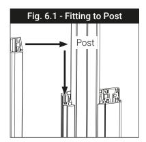
For a panel, overlap the extrusions and slide it down the post. For a door, apply a thin layer of clear silicone to the mating face of the bottom pivot block. Attach it with a  $3.5 \times 25$  mm pan head screw (No.6 x 1") and then slide the door down the post.
