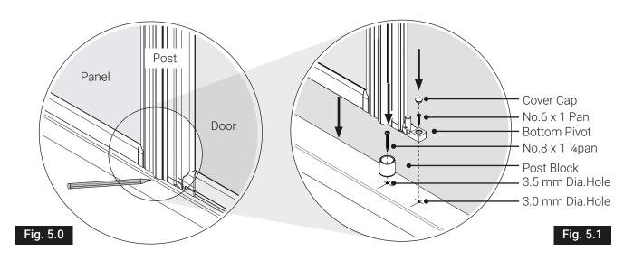
Mark and drill the screw hole positions. NB, the holes are different sizes. Screw the post block down with a  $4.2 \times 32$  mm pan head screw (No.8 x 1 ¼"). Replace the post and door, then screw the pivot block down with a  $3.5 \times 25$  mm pan head screw (No.6 x 1").
