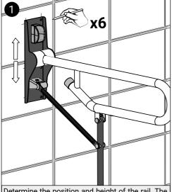
Determine the position and height of the rail. The rail must be level when in the down position and the leg must be vertical. Mark the hole positions on the wall through the mounting plate.
