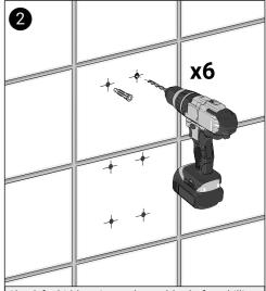
Check for hidden pipework or cables before drilling. Use Masking tape to protect tiles from splintering. Drill suitably sized holes for the fixings being used. Insert wall plugs. Fixing not supplied.
