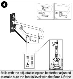
to make sure the foot is level with the floor. Lift the cover (D) and unscrew the adjustment foot (C) until it is tight against the floor. Lock the foot with by tightening the nut up with a spanner. Then slide the cover back down. Check the levels.
