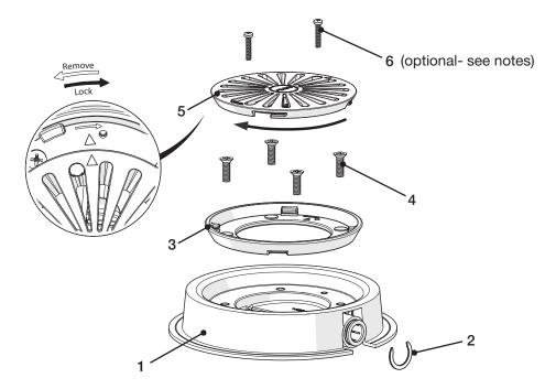
Install the wet-floor covering ensuring all of the manufacturer's instructions are followed. Trim the wet-floor covering to fit the Screedmaster opening and align and fit the clamp ring (3) with qty 4 M6 stainless steel screws (4).
