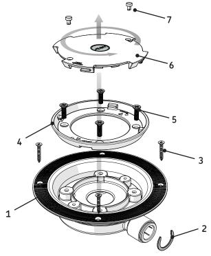
Install the wet-floor covering ensuring all of the manufacturer's instructions are followed. Trim the wet-floor covering to fit the Silentflow $^+$  opening and align and fit the clamp ring (4) with qty 4x M6 stainless steel screws (5).
