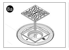
Temporarily cover the waste whilst tiling to prevent tile adhesive entering the waste.
