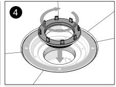
Screw the waste retaining ring to the waste body until it creates a water tight seal.
