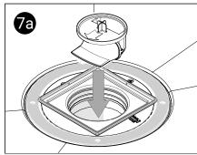
Lower the dry trap into the waste main body making sure that the valve faces towards the waste outlet pipe.
