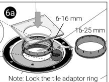
Depending on the thickness of your tiles select either 6-16 or 16-25 mm tile height adjuster ring.
