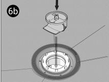
Lower the dry trap into the waste main body making sure that the valve faces towards the waste outlet pipe.
