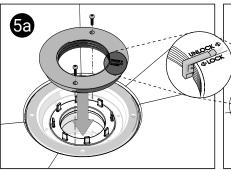
Secure the locking ring to the waste adaptor with the screws.
