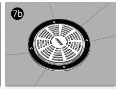
Whilst work continues in the area. Temporarily cover the waste area to protect the trap from any debris entering. Once complete attach the safety floor waste cover ensuring the location pegs are inserted into the clamping ring.
