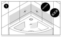
Ensure that the washbasin is level and mark the desired fixing location using the holes in the washbasin as a guide.
