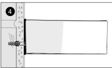
Secure the washbasin to the wall and do not over-tighten fixings. Remove any excess sealant. Fit the tap and waste pipe in accordance with the manufacturer's instructions.
