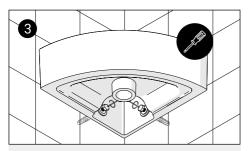
Offer the basin up to the wall. Ensure washbasin is level before tightening the wall fixings. Apply sealant around the washbasin and wall.
