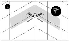
Drill holes and insert the wall plugs.
