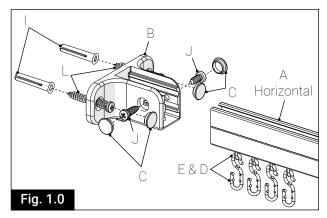
Fixing Screws (L - No.8 x  $1\frac{1}{2}$ " pan). Lightly spray rail with silicone lubricant to help Ceiling Hanger Bracket (G) to slide in to the top section of the rail and the Gliders (E) in to the bottom section of the rail. Insert the rail into the wall brackets and secure with Small Screws (J - No.8 x  $\frac{1}{2}$ " pan). Fix Screw Cover Caps (C).
