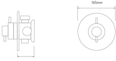
65mm min, 70mm max from back face of valve to finished / tiled wall surface (10mm allowance for tiles)
