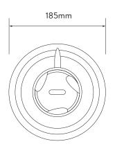
Distance from back face of valve to finished wall surface (includes 10mm allowance for tiles) MIN 60mm, MAX 100mm
