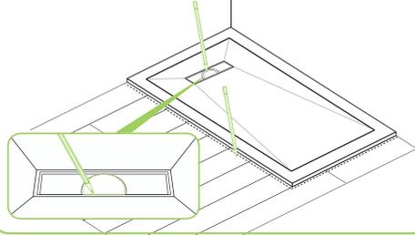
Take care to avoid chipping on bottom edges/corners when moving the tray into position.
