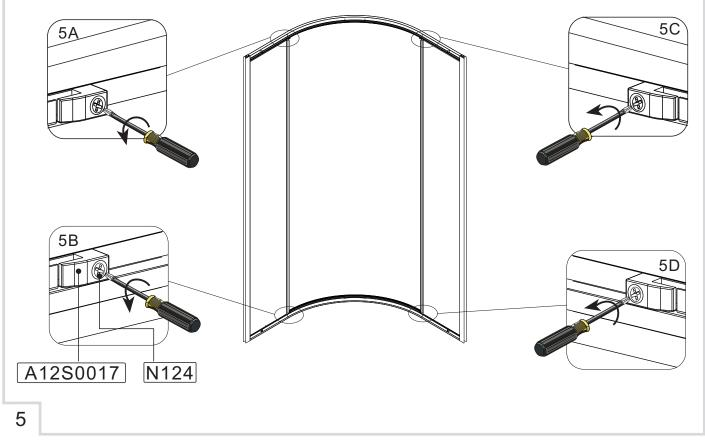
Slot the top and bottom profile fixing screws into the slots in the upright profile.
