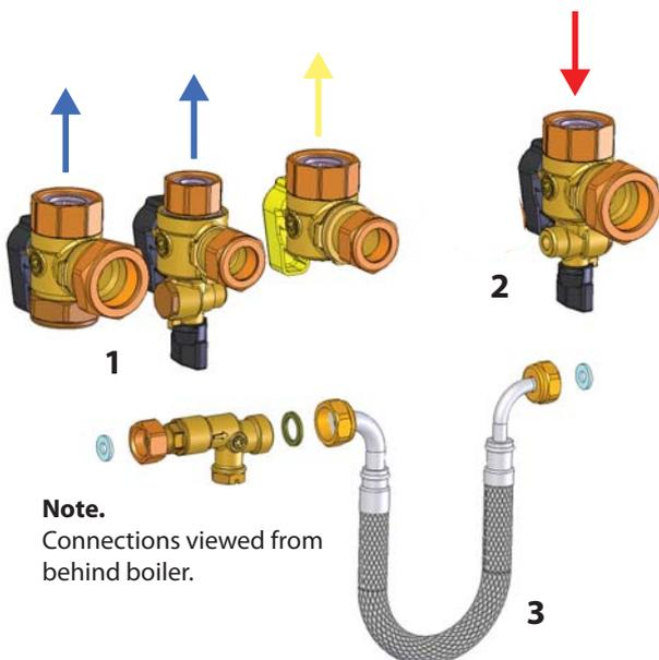
1. To repressurise the system ensure flexible hose 3 is connected
