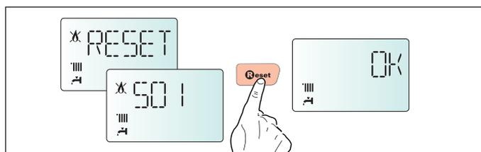
**IF THIS SHUTDOWN OCCURS FREQUENTLY, CONTACT AN AUTHORISED SERVICE CENTRE FOR ASSISTANCE. FOR SAFETY REASONS, THE BOILER WILL ALLOW A MAXIMUM OF 5 RESET OPERATIONS TO TAKE PLACE IN 15 MINUTES (INDIVIDUAL PRESSES OF THE **Reset** BUTTON).**
