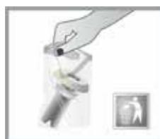
Dispose of the used cartridge into regular household waste.
