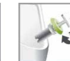
Using the Service Key, screw the cartridge clockwise into the cartridge holder until the cartridge sits evenly.
