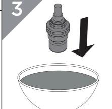
Place valves in a suitable solution and soak until fully de-scaled.
