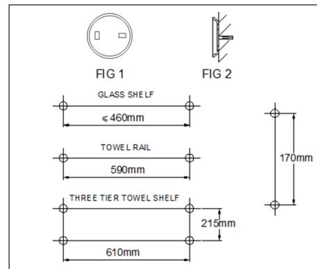
**NOTE:** All dimensions refer to the pillar centers. Guide dimensions only. All centers should be measured and checked prior to drilling.
