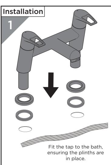
Secure the taps to the bath by using the washer and metal backnut below the bath.
