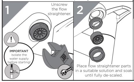
Reverse the maintenance steps to replace the flow straightener.
