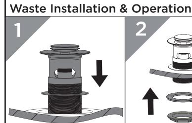
Fit the waste above the basin ensuring the washer is in place.
