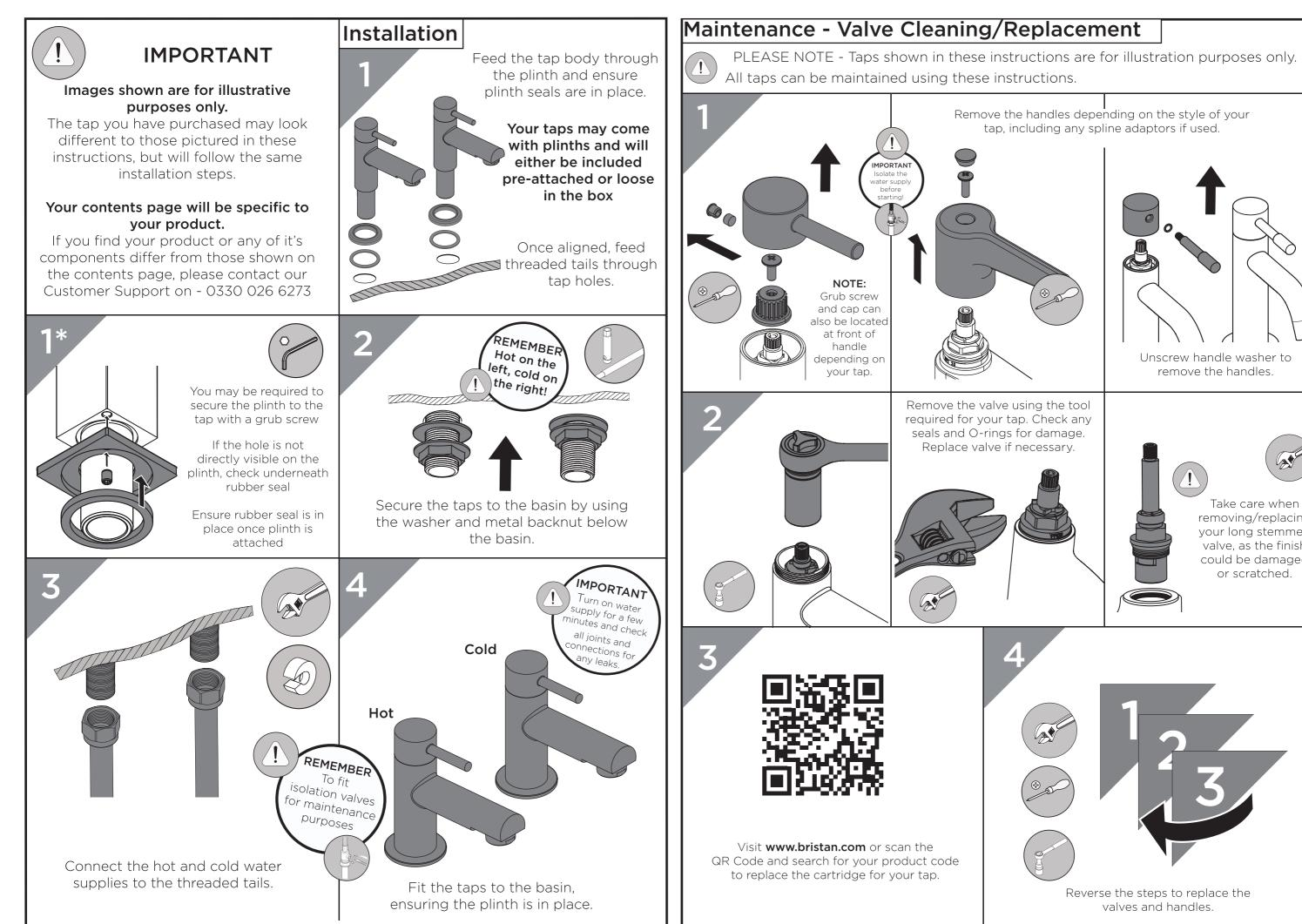
Remove the handles depending on the style of your tap, including any spline adaptors if used. Unscrew handle washer to remove the handles. Take care when removing/replacing your long stemmed valve, as the finish could be damaged or scratched. Reverse the steps to replace the valves and handles.
