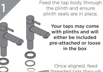
Once aligned, feed threaded tails through tap holes.
