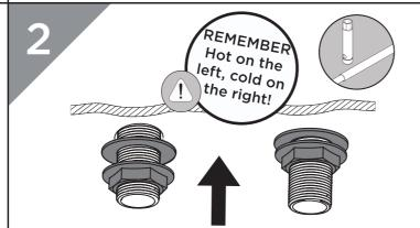
Secure the taps to the basin by using the washer and metal backnut below the basin.
