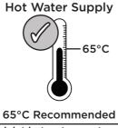
The inlet hot water must be at least 10°C above the required blend temperature.
