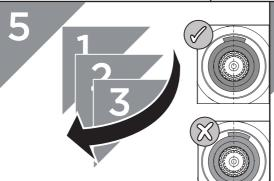
Reverse the installation steps, ensuring the temperature stop is aligned correctly.
