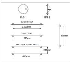
**NOTE:** All dimensions refer to the pillar centers. Guide dimensions only. All centers should be measured and checked prior to drilling.
