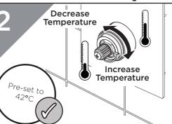
Turn the spindle to increase or decrease the temperature. Check the temperature and adjust until you achieve the desired result.
