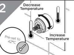
Turn the spindle to increase or decrease the temperature. Check the temperature and adjust until you achieve the desired result
