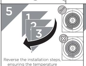
stop is aligned correctly.
