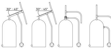
Off expansion pipe with rising 28mm offset reducing to 22mm pipework to pump and expansion pipe. Off expansion pipe with rising 22mm offset and 22mm pipework to pump. Top Entry flange (Part No 27800) with 22mm pipework to pump.
