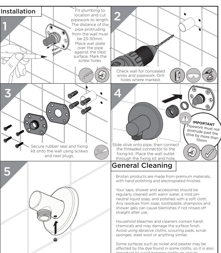
Secure in place with grub screw. Screw the shower hose (not supplied) onto the outlet ensuring the sealing washer is fitted.
