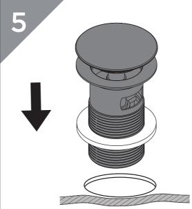
Feed the waste body through the basin, ensuring the rubber washer is in place.
