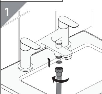
Secure nut end of hose onto the threaded outlet connection, ensuring the washer is in place before securing
