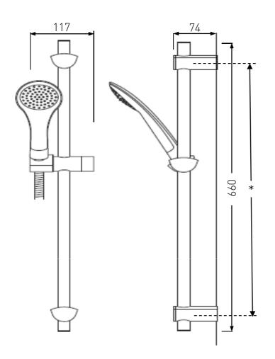
\* Note: The Riser rail wall brackets can be positioned up or down the riser rail as required. This allows any existing holes to be reused or covered by the wall brackets. The brackets can also be adjusted to sit in the middle of the tiles or in the tile joints. EV KIT02 C
