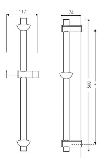
\* Note: The Riser rail wall brackets can be positioned up or down the riser rail as required. This allows any existing holes to be reused or covered by the wall brackets. The brackets can also be adjusted to sit in the middle of the tiles or in the tile joints.
