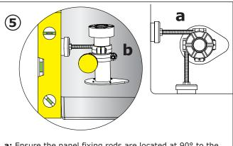
${f a}{:}$  Ensure the panel fixing rods are located at 90° to the edge of the tray as shown above.
