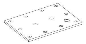
Turn the tray over and use the cardboard packaging as a protective mat. Note the circles that have been marked to indicate feet position. The symbol  $\bigoplus$  indicates where you should fix the feet with the panel fixing rod, but for the symbol  $\bigoplus$  you will only use five of these positions and the other three would be supplemented with the feet without the panel fixing rod.
