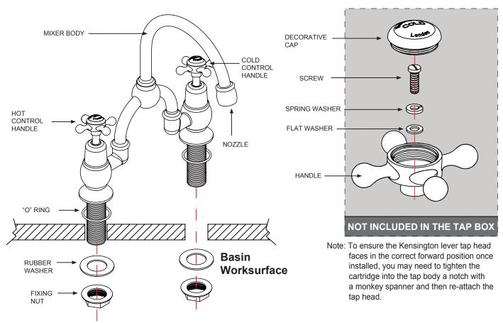
A) Fit the "O" ring into the groove on the underside of the tap body.
