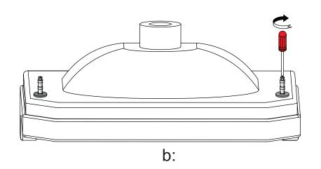
(4) Refit the rail to the connectors and lock in position with the 4 grub screws.
