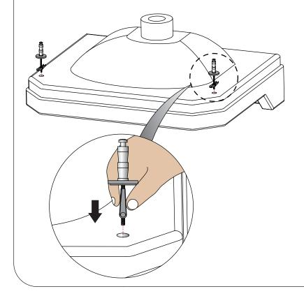
2 Pull the fixing bolt up so that it catches on the inner surface of the basin, and then tighten, but only tight enough to prevent the fitting sliding too much.
