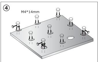
Screw the feet in position with the screws provided. Ensure that the foot that has two panel fixing rods attached, is placed in the corner where the panels will
