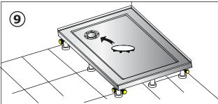
When shower tray is set remove the remainder of the protective plastic film and connect the waste pipe and check for leakage and water drainage.
