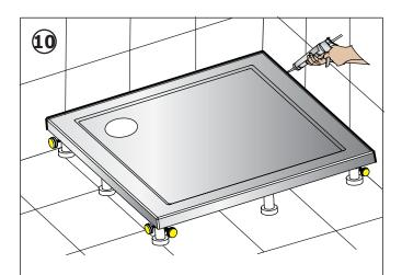
Tile the wall and seal joints with an anti fungal silicone sealant and allow to set.
