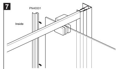
Push fit the vertical seal (PN40331) onto the back edge of the door, the curved flap **must** be positioned as shown.
