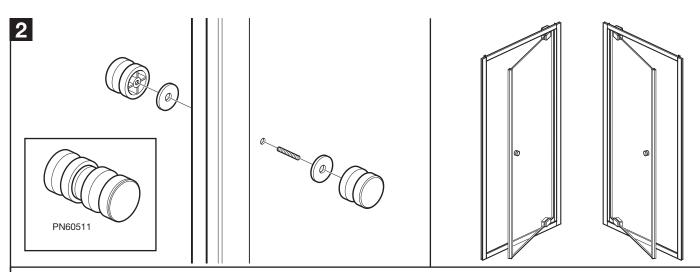
Fit the door handle to the door ensuring the plastic washers are fitted each side of the glass. Choose the opening side for the door (turn over if necessary).
