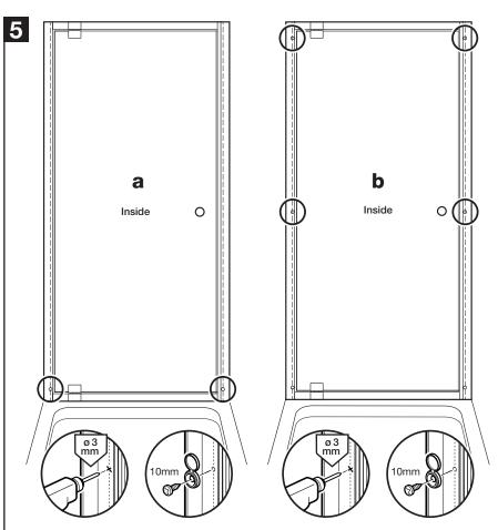
Check door is centrally positioned, perfectly vertical and square in the frame.
