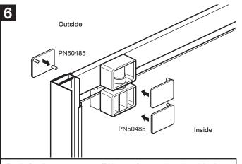
Push fit all 6 cover caps (PN50485) onto the pivot blocks at the top and bottom of the door (inside and outside).
