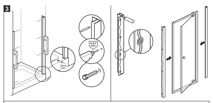
Place wall channels on tray ensuring they are vertical and a minimum of 3mm back from the front of the tray. Place masking tape against the wall before marking the drill hole positions. This will prevent the drill bit slipping. Drill 6.5mm holes, 30mm deep and insert wall plugs.
