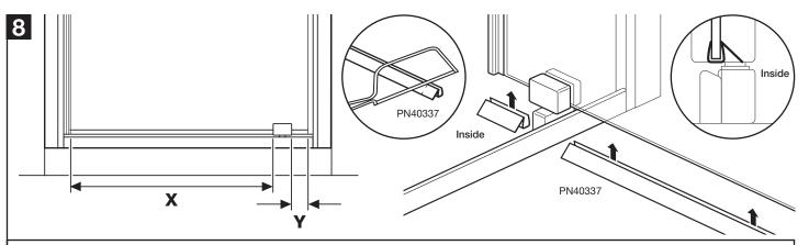
Measure dimensions 'X' (from magnetic seal to pivot block) and 'Y' (from pivot block to vertical seal). Cut horizontal seal (PN40337) to the lengths measured using a hacksaw. Push fit cut seals onto the bottom of the door, the seal 'flap' must be on the inside. Note: Wetting the edge of the glass will help the seal fit.
