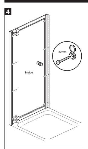
Place door in position on the tray, fix wall channels to the walls (in all 8 positions shown) using 32mm screws and screw caps.
