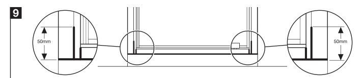
From the outside only, apply sealant to the bottom of the enclosure and 50mm up the wall channels as shown.
