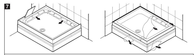
Peel back protective film from back edges of tray. Tile over the upstands. Seal the wall edges of tray with silicone sealant. When the final installation of the enclosure is complete, remove the remaining protective film.
